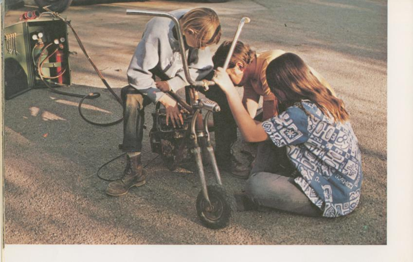
If you know how to *weld* you can build your own minibike. After the frame is welded together, you put on the wheels, handlebars, brakes, and seat. Then all you do is hope all the parts stay together while you ride.
