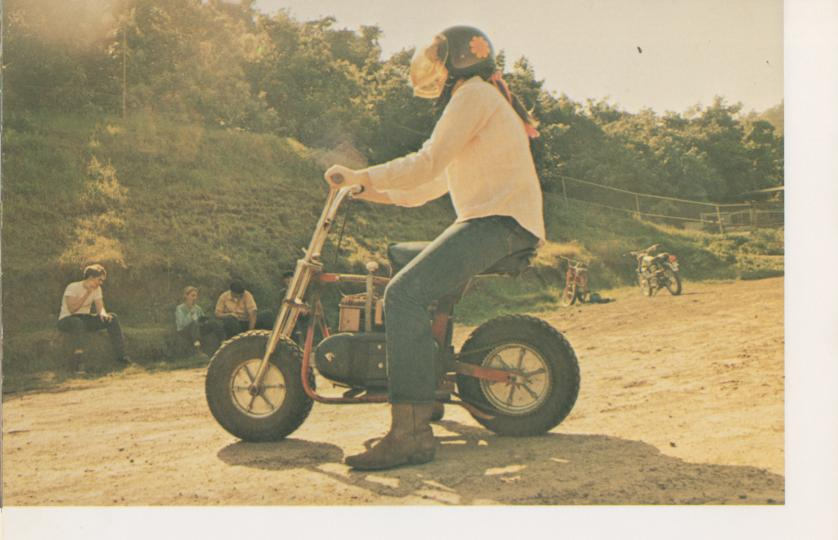
No matter where a minibike is built, it must have certain parts. The main part, the *frame*, holds the seat, engine, rear wheel, and *front fork*. The handlebar and front wheel go on the front fork.
