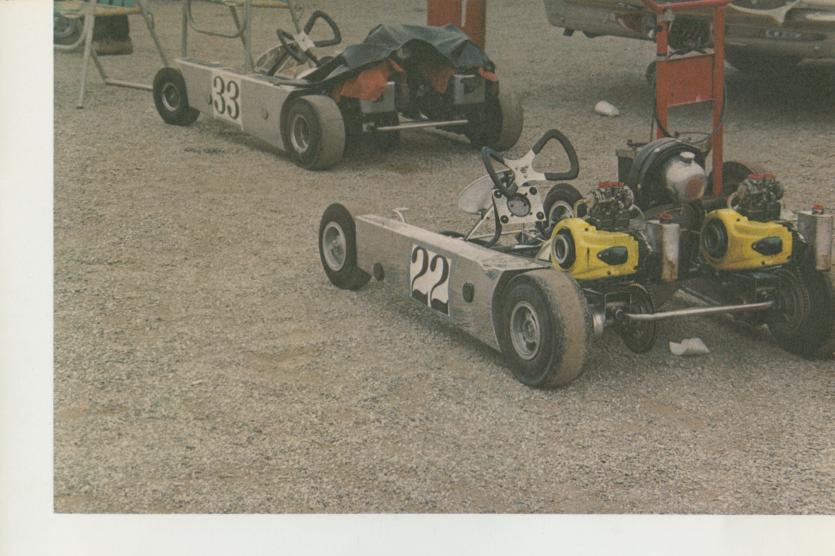
Enduro karts carry side tanks of fuel for the long race. As in all karting, races are run in classes. Enduro regulations set classes according to number of engines, driver's age, and total weight of driver and kart.
