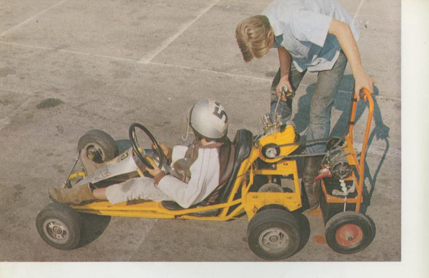
The best way to start kart engines is with a batteryoperated electric motor. First you squirt some fuel into the carburetor for a prime start. Then the electric motor gives the engine a spin to get it running.
