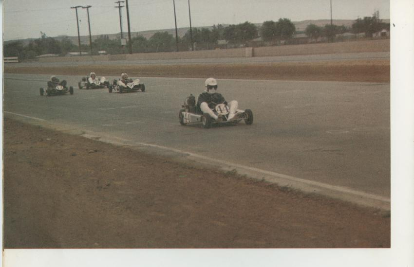
Because of long straightaways and engine gearing, enduro karts reach speeds above 120 miles per hour. Some enduro karts are built so the driver can lie down to keep the weight close to the ground for better cornering.
