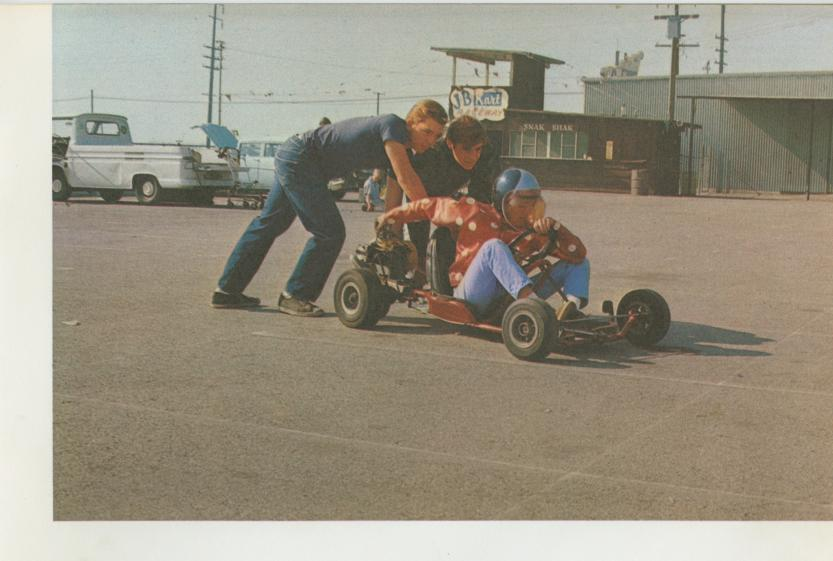
This driver gets his friends to give his kart a push start. His hand on the carburetor chokes the engine to make it suck more fuel. When the engine starts, the driver stops choking and the friends stop pushing.
