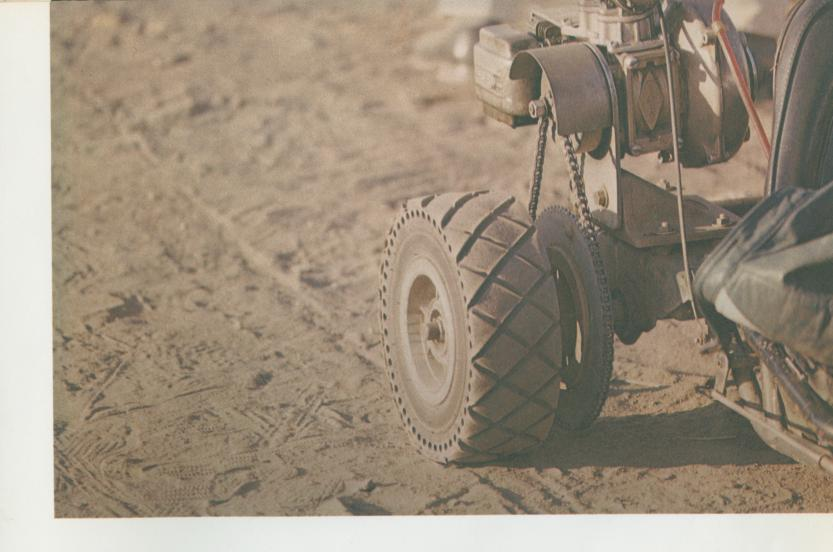
When the dirt on the track is soft, drivers use a different tire to get a better bite. This tread allows just enough slip, so the kart can slide around the turns.
