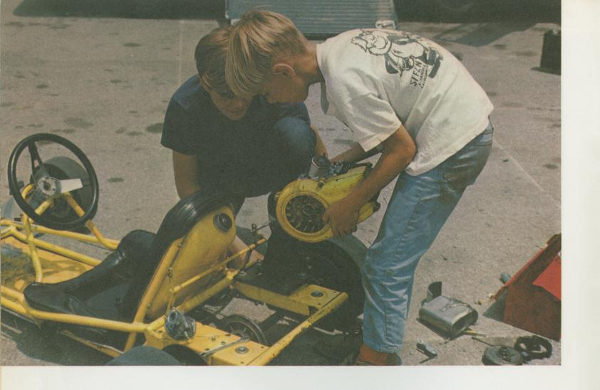
High-speed, two-cycle karting engines need many repairs. In spite of their power, these engines weigh only about ten pounds. A good mechanic can remove an engine in less than fifteen minutes.
